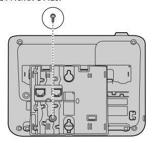
**3.** Connect the cables to the unit, and run the cables through the wall mounting adaptor, as shown in the illustration below.
