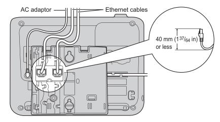
**4.** Drive 2 screws into the wall as shown in the illustration below, and mount the unit on the wall.
