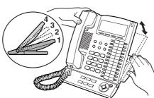
The tilt angle of the operation board can be adjusted to one of four angles.
