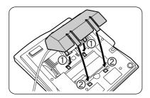
Pull down the handset hook until it locks, so the tab holds the handset.
